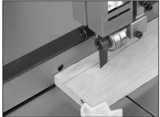
Figure 62. Blade leading away from line of cut.
